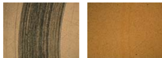
Fig. 23: Pin-on-Disk test of PMMA on TiN coated substrate.
