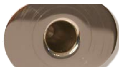
Fig. 11: Scratched non-coated CoCr tibial component
