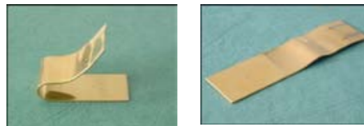
Fig. 24: Bending test to prove adhesive strengths
